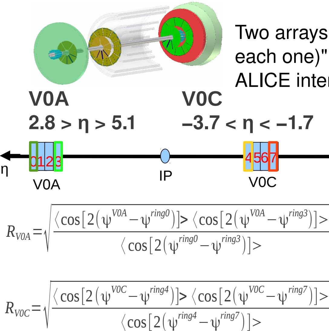
Two arrays of scintillator counters "(4 rings each one)" installed on each side of the ALICE interaction point.
