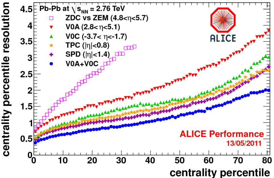
The best centrality accuracy is provided by VZERO: from 0.5% in most central to 1.5% in most peripheral events
