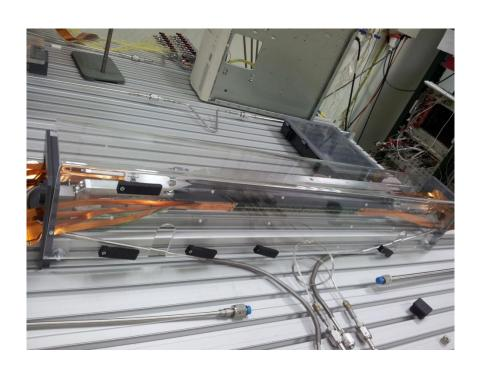
Set up one of the two lines of the DSF cooling plant to allow the characterization of the SPD spare sector.
