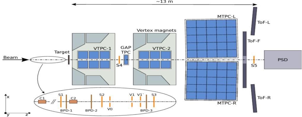
Beam detectors and triggering → A set of upstream scintillation or Cherenkov counters and beam position detectors, provides precise timing reference, charge and position measurement of the incoming beam particles
