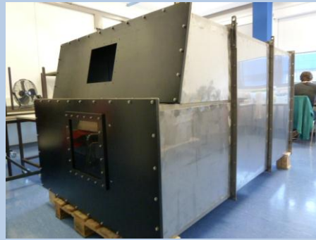
Proximity-focusing RICH with granular MAPMT readout
