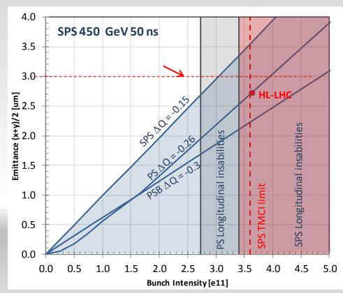
Limited by longitudinal instabilities in PS and SPS, and by brightness in SPS
