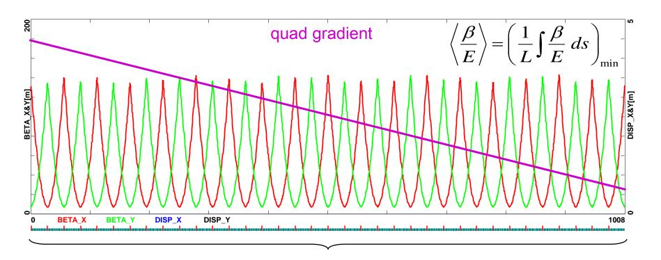
17 FODO cells (17  $\times$  2  $\times$  16 = 544 RF cavities)
