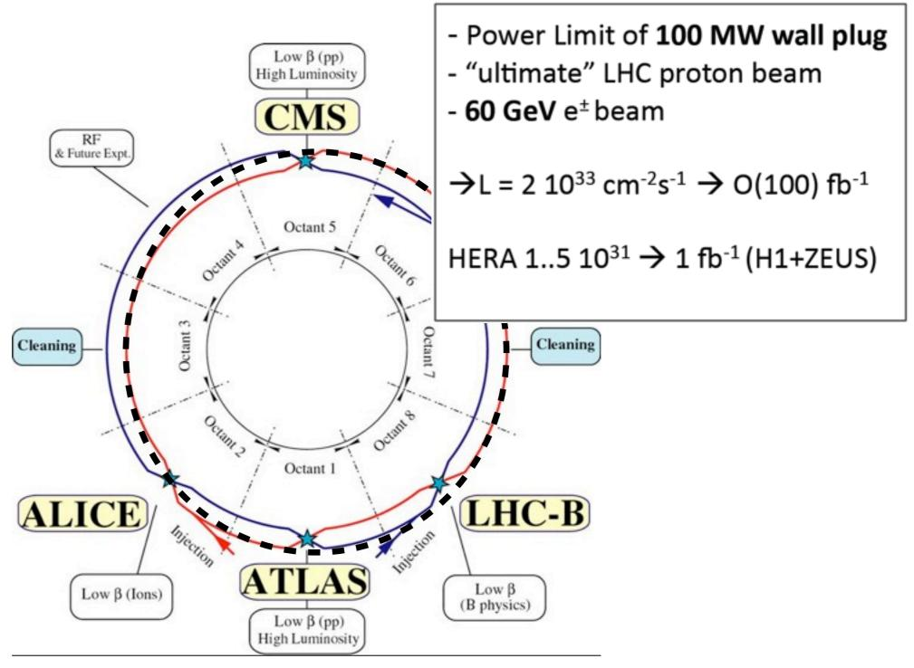
Either by installing a new electron storage ring in the LHC tunnel (Pol~40%)
