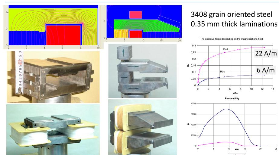
After cycles of different amplitude, the remanent field is of about 1 Gauss in all cases. The measured reproducibility of the injection field is about  $\pm$  0.075 Gauss.
