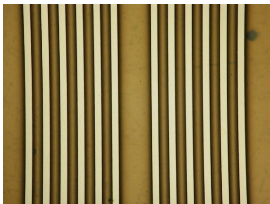
15 μm line/space conductors
