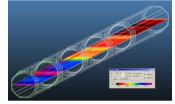
The integrated flux along the ~ 7700 mm-long orbit is F=2.84E+17 ph/s, and the integrated power is P=0.88 W, for the nominal HiLumi current of 860 mA.
