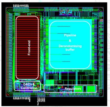
Design of the ABCN-25 ASIC for readout of silicon microstrip detectors. (CERN. AGH Kraków, U. Geneva, U. Penn)
