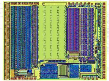
128 front-end channels2 levels of data bufferingData derandomization and zero supressionRadiation hardness up to 10 Mrad
