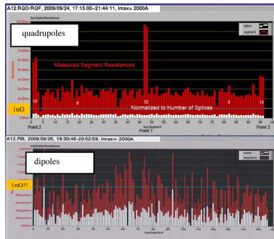
Fig. 18. Measurements of the resistance of the sc inter-magnet splice resistances (white lines are the calculated resistances of the splices).
