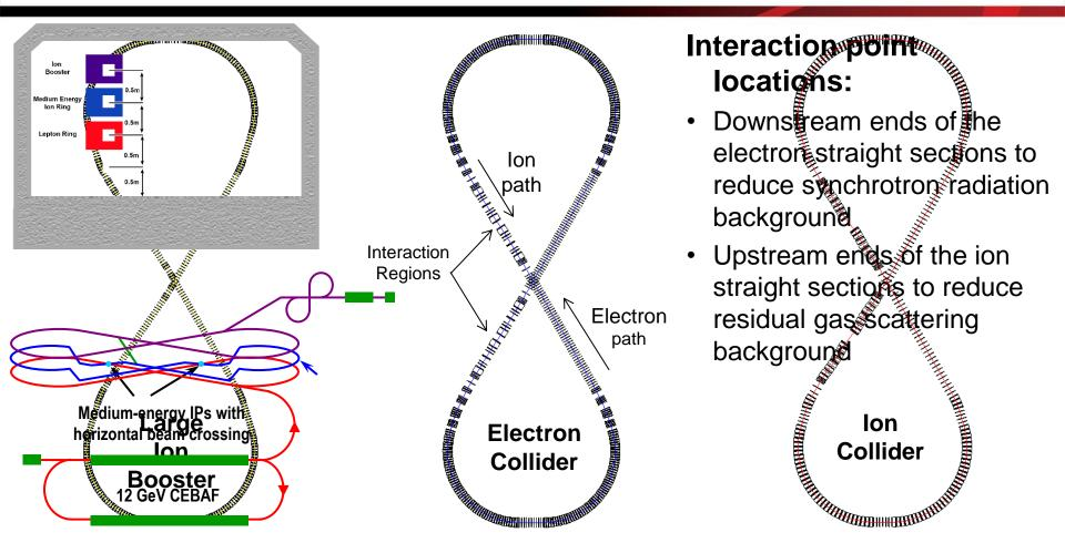
• Vertical stacking of nearly identical rings (max. deviation: 4 m; ring circumferences: 1350 m)
