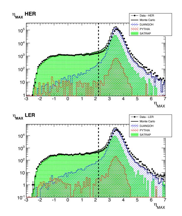
**Figure 5.10:** The  $\eta_{MAX}$  distributions for the DIS HER (up) and LER (down) inclusive data samples. The histograms represent the sum of the Monte Carlo contribution: non-diffractive DIS (DJANGOH) is the blue histogram, photoproduction (PYTHIA) is the red one and diffractive events (SATRAP) are shown in green.
