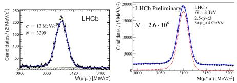
• Signal peaks fitted with Crystal Ball functions.
