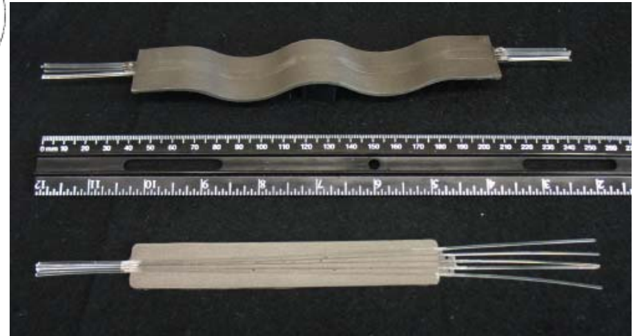
Scintillating fiber in tungsten powder epoxy polymer
