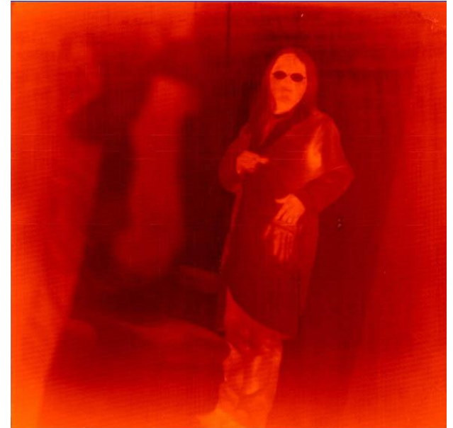
8-12 \mu\text{m} IR image taken with NASA 1 megapixel GaAs QWIP
