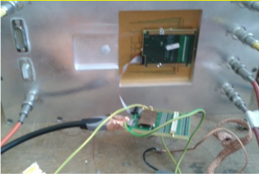
APV mounted on the anode
