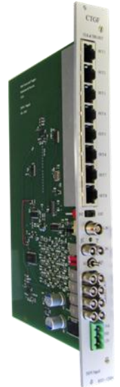
SRS: CTF card Clock, Trigger and IO
