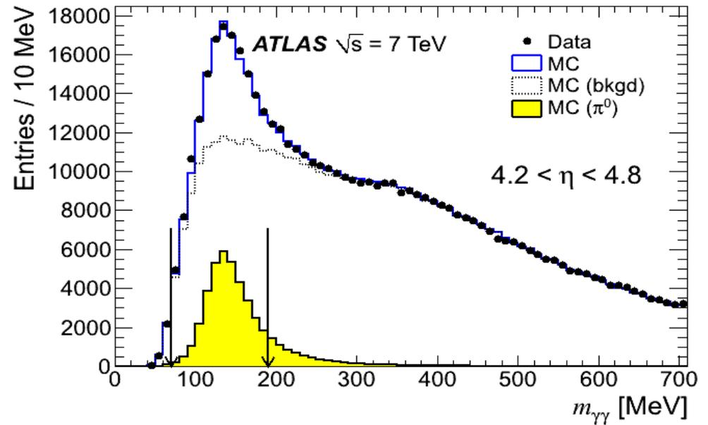
Figures showing  $\pi^0 \rightarrow \gamma\gamma$  resolution in both the central and forward regions.
