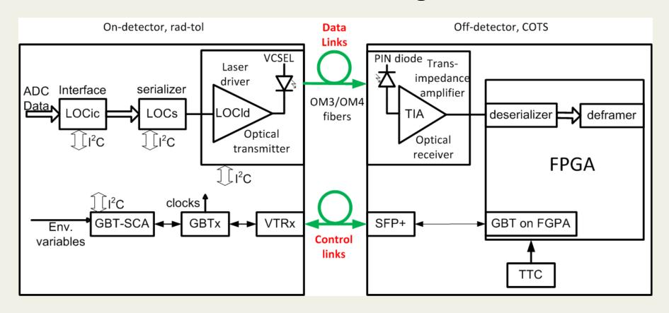
The ASIC approach, based on LOC and GBT+VTRx
