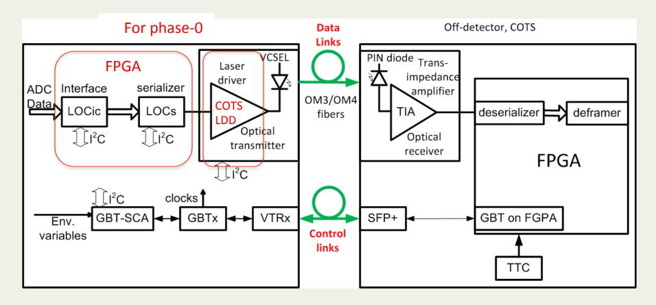
For phase-0 (or LS1, 2013/14) installation, as a demonstrator for system proof-of-principle, Kintex-7 and COTS LDD will be used in places of LOC ASICs.
