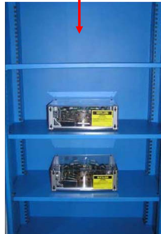
Dry box for half disks storage at CERN
