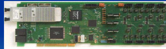
Floor Control Module: 1° level concentrator
