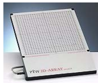
729 ionization chambers 27x27 cm 2 Pitch 10 mm
