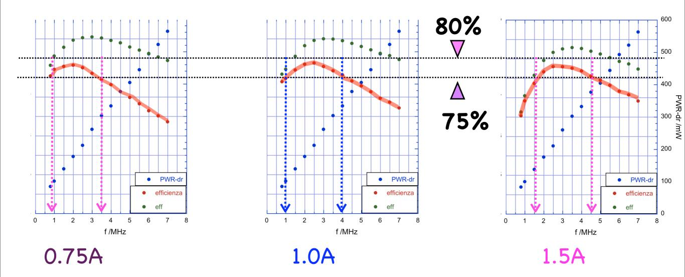
Drivers power: 5 mW/ (MHz x gate) -7% -1MHz ...frequency position of the maximum efficiency
