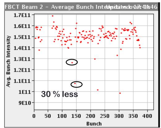
12 + 144 bunches at injection in the LHC: Problem with injection kicker timing in the SPS
