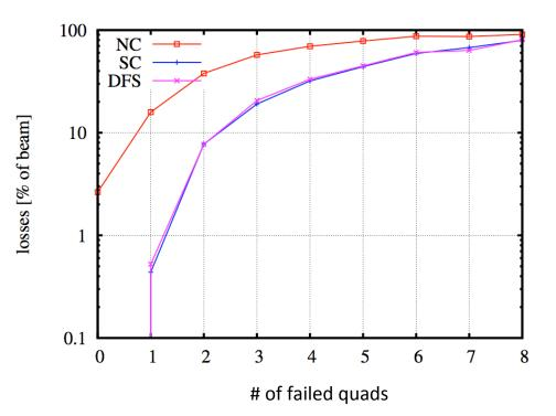
Simulation of Failure modes for uncorrected machines (NC), 1:1 steered machines (SC), and DFS steered machines (DFS)
