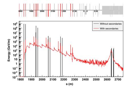
Energy deposition along the beam line from halo particles, with (red) and without (black) secondary particle production and scattering. Losses from synchrotron radiation have not been included.
