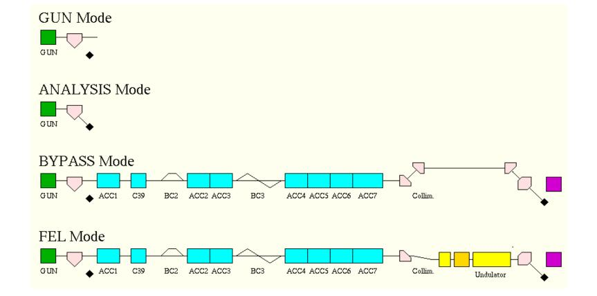
MPS determines operation mode from machine settings
