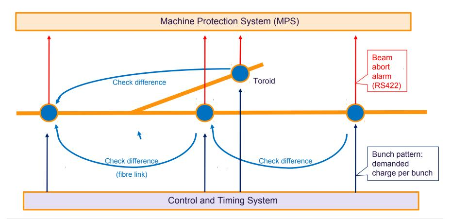
"Toroid Protection System" (TPS) is one application of the Toroid system:
