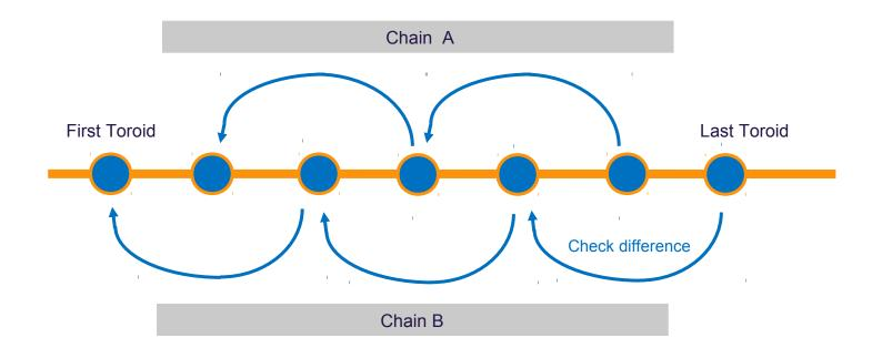
Redundancy for the TPS functionality is added by interleaved fibre chains.
