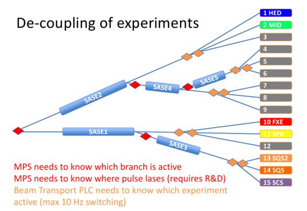
15 experiments in 5 SASE beamlines, 5 experiments with different beam requirements operated at the same time
