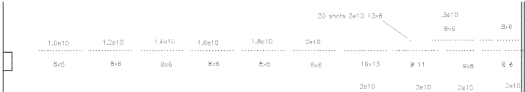
Figure 2: Sketch of a section of the copper coupon showing beam impact points (IPs) and associated parameters. The coupon size is 15.54 x 13 mm.
