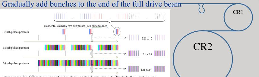
Three cases for different number of sub pulses per decelerator train to illustrate the resulting non continuous bunch structure of the decelerator trains.
