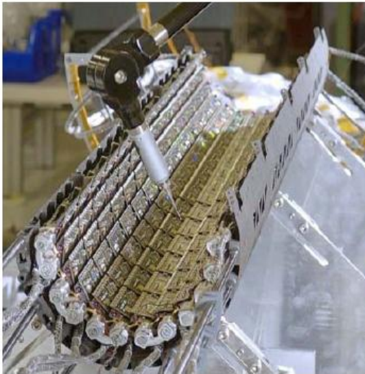
1744 Pixel modules, pixels 50 \times 400 \mu\text{m}^2
