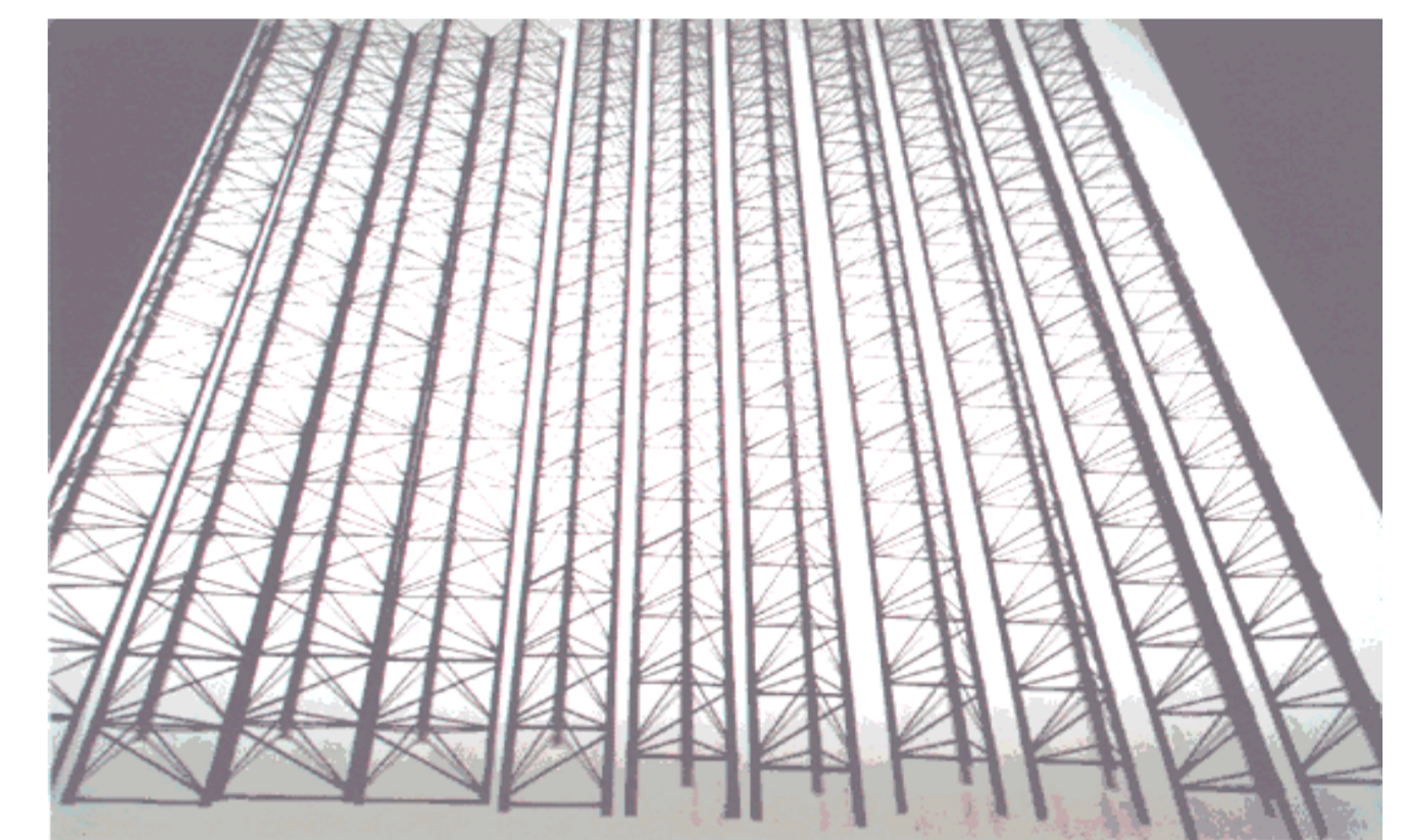
Ultralight (22g, L=1.1m) CF space frames produced in St.Petersburg for the currently running ALICE/ITS
