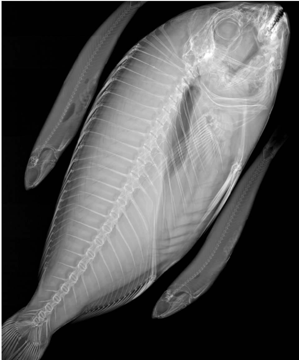
A large area (25x20 cm 2 ) image of a sea-bass fish and two anchovies taken in slot-scanning mode and a detail of mouth and teeth
