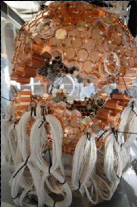
XMASS at Kamioka: in water Cherenkov shield at Kamioka 835 kg LXe (100 kg fiducial), single-phase, 642 PMTs soon to take science data
