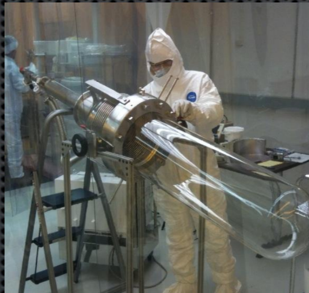
COUPP 60 kg CF 3 I detector installed at SNOLAB; physics run in March 2013
