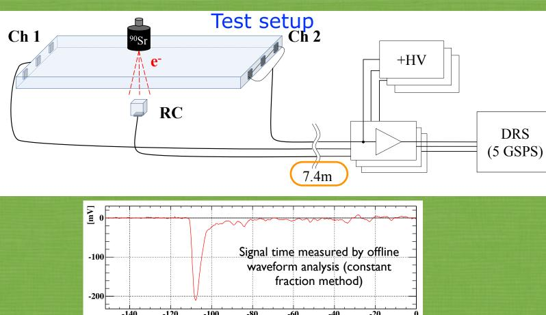
Single pixel time resolution Best time resolution 42ps obtained at optimum over-voltage of 2.3V/MPPC
