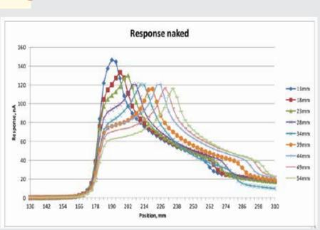
**Normalized Response of Tiles with Groove Displacement (3.2mm Scintillator without Wrapping)**
