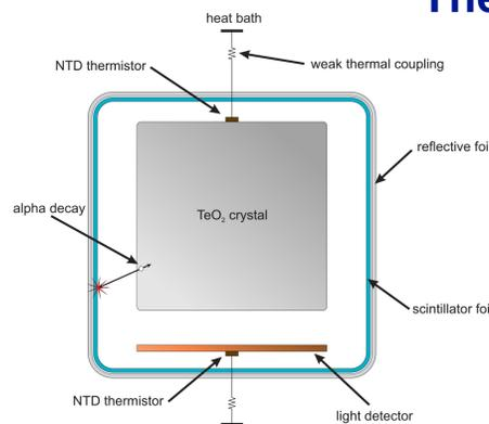
To tag the events coming from surface contaminations the thermal detector can be encapsulated in a scintillating foil. Adding a bolometric light detector, should make possible to detect the light produced by the interaction of degraded  $\alpha$  particles with the scintillating foil.
