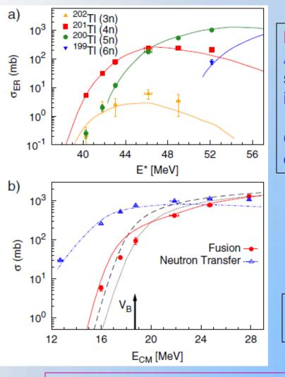
**Evaporation residues from CN**<sup>205</sup>**TI** Accuracy similar to stable beams for low xsec at sub-barrier: first time with low intensity RIB
