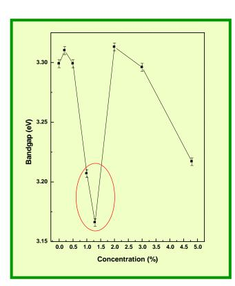
⇒ The band gap of pure ZnO is ~ 3.3 eV, which is in agreement with the band gap of ZnO prepared by other techniques [Appl. Phys. Lett. 65 (1994) 1373]
