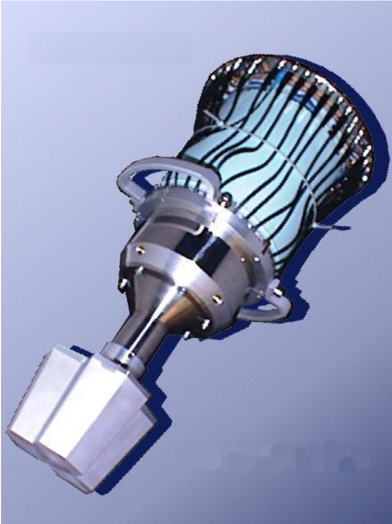
Triple cluster detector 3 x core + 3 x 6 segments IKP Köln and CTT
