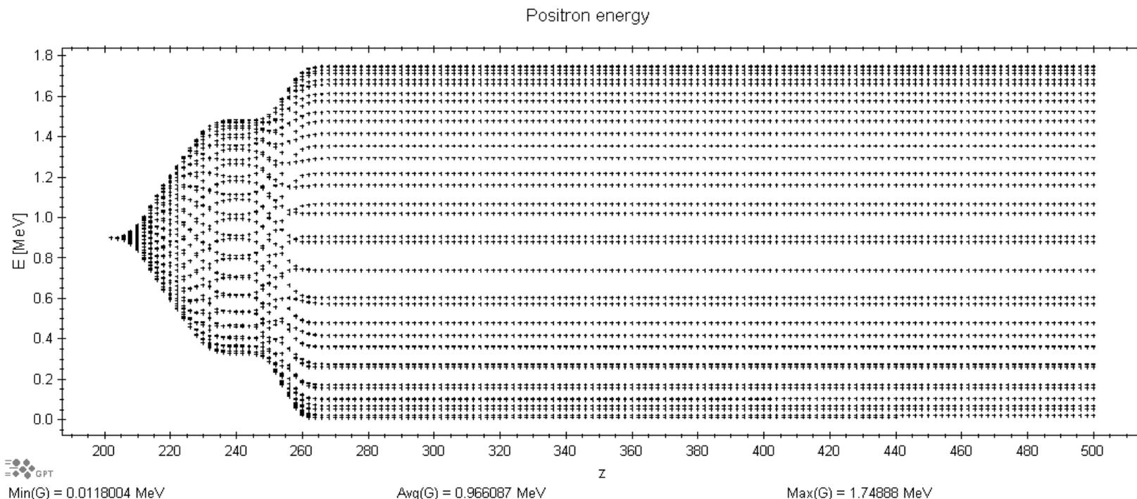
Deceleration and acceleration by 2 RF cavities
