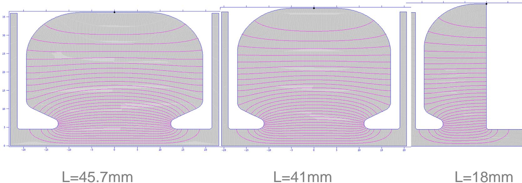
Different positions of cavities and focusing solenoid were tested.
