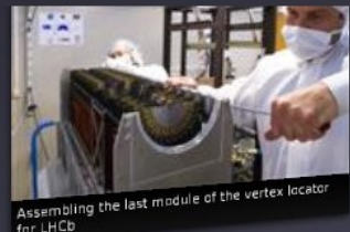
Assembling the last module of the vertex locator for LHCb
