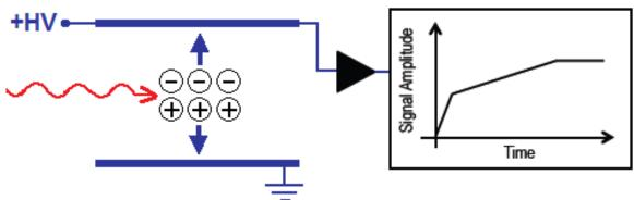
2. Ion Mobility Spectrometry → Technique that aims at identifying ionized molecules in a gas based on their mobility in a carrier buffer gas.
