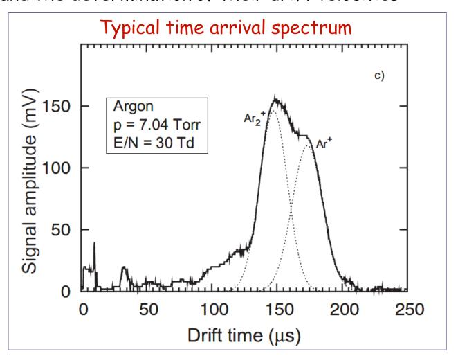
The drift-time spectrum shows two distinct peaks, corresponding to two types of ions with different mobilities
