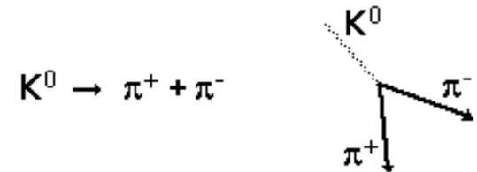
$$\begin{aligned} m^2 &= E^2 - p^2 = (E_1 + E_2)^2 - (\mathbf{p}_1 + \mathbf{p}_2)^2 \\ &= m_1^2 + m_2^2 + 2E_1 E_2 - 2\mathbf{p}_1 \cdot \mathbf{p}_2 \end{aligned}$$
