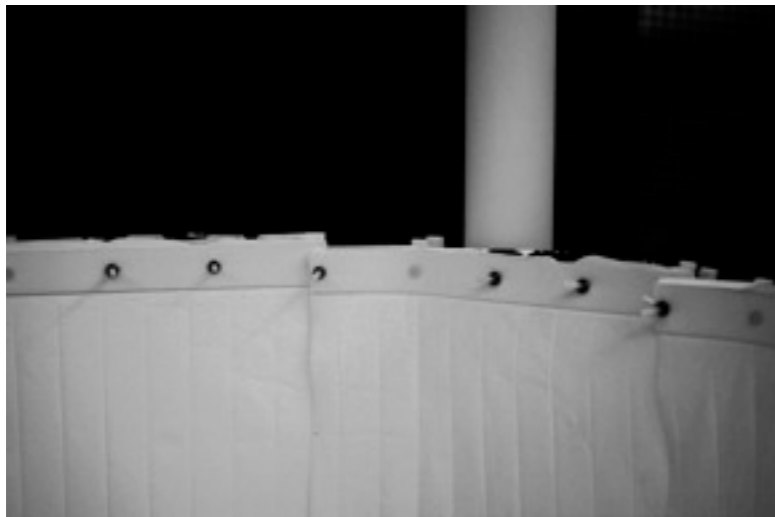
Reflector foils mounted on field cage
