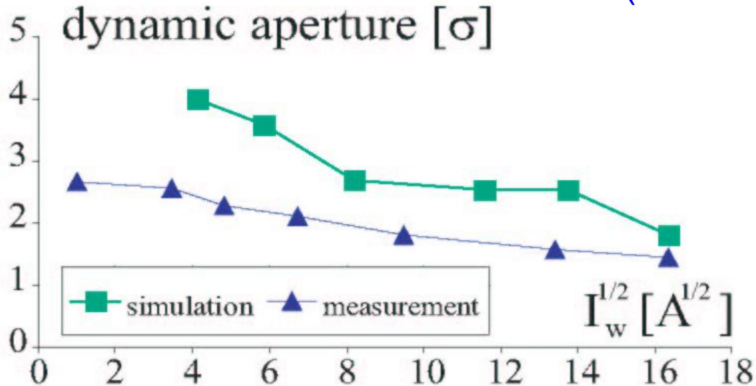
*linear dependence  $DA(I_w^{1/2})$  consistent with Irwin scaling law; measured dynamic aperture is smaller than simulated*
