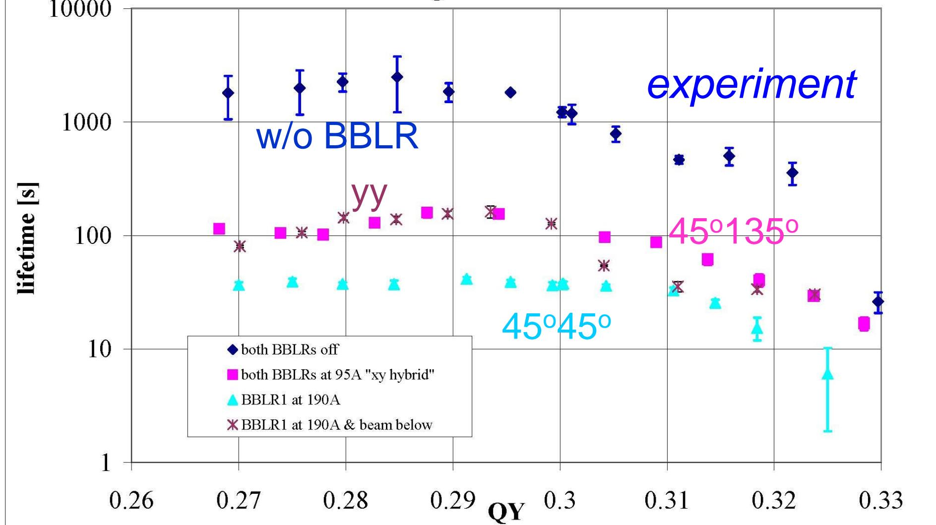
*measured beam lifetime is worst for ' $45^\circ 45^\circ$ ' crossing, and at tunes above 0.3 best for ' $45^\circ 135^\circ$ ' crossing*
