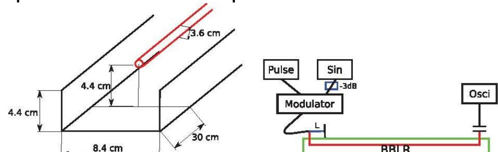
(a) Dimensioning of the RF-BBLR prototype # 2
