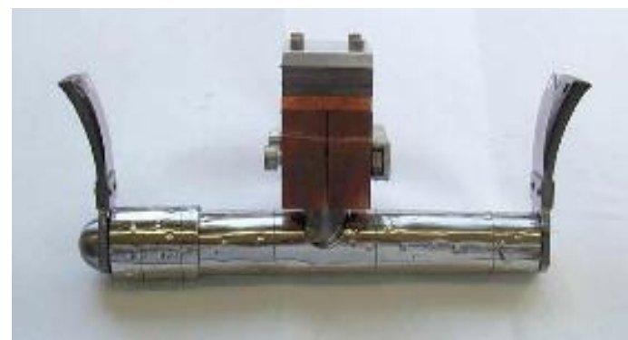
Pb/Bi264 container after dismantling in 2007
