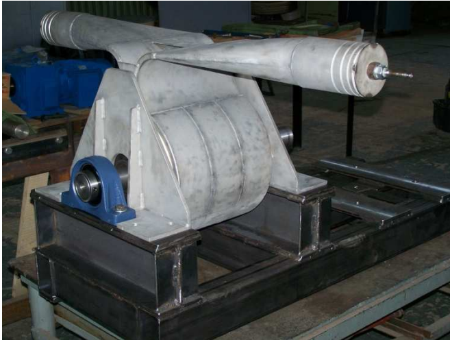
PbBi pump - developed P = 6 bar, provided flow rate Q = 7 L/s.
