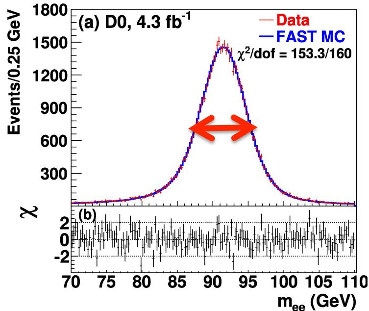
$$\sigma_{\text{observed}} = \sigma_{\text{detector}} \oplus \Gamma_Z$$
