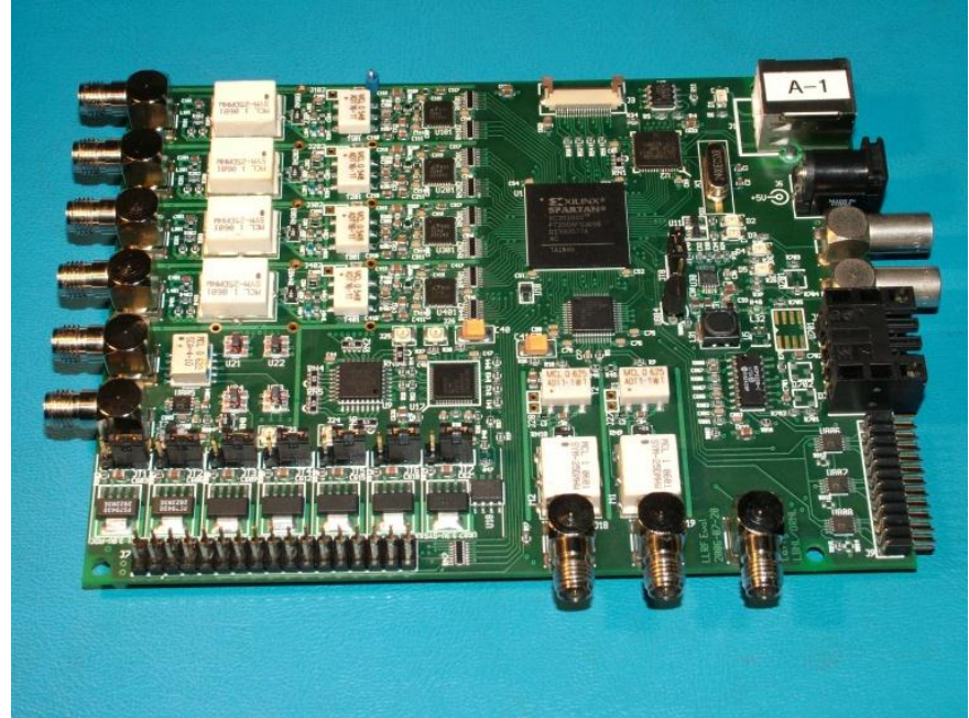
1.3Ghz feedback system on ALICE
